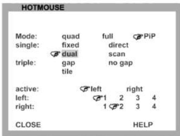
**Single dual:** The left half of the first channel is displayed at full size next to the left half of the second channel.
