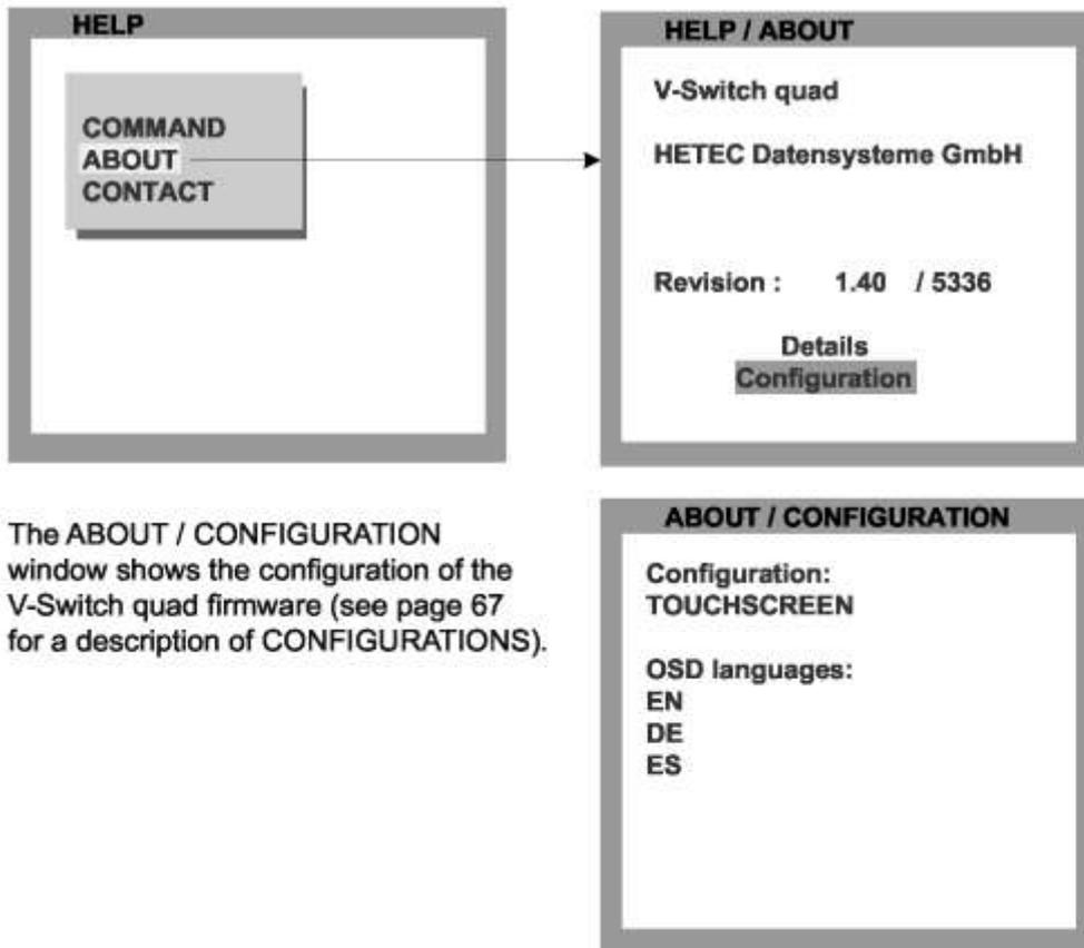
The ABOUT / CONFIGURATION window shows the configuration of the V-Switch quad firmware (see page 67 for a description of CONFIGURATIONS).
