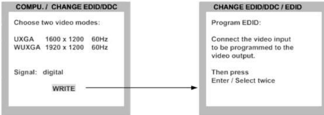
When the window shown on the right opens, connect the video output to the video input to be programmed with a DVI video cable.
