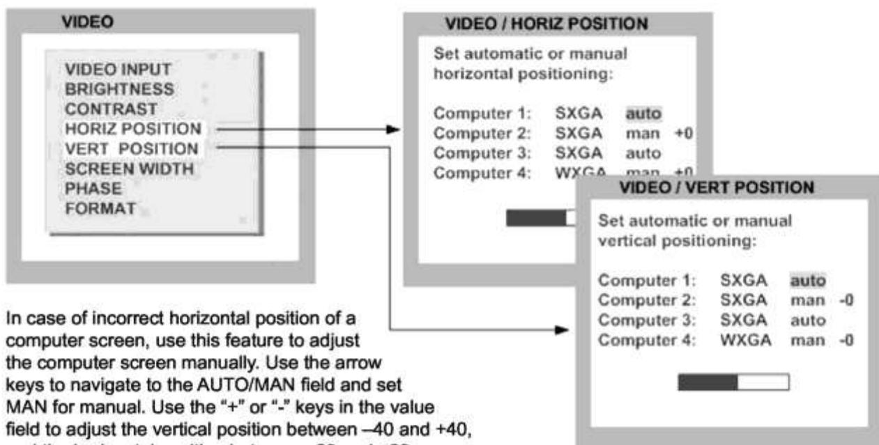
In case of incorrect horizontal position of a computer screen, use this feature to adjust the computer screen manually. Use the arrow keys to navigate to the AUTO/MAN field and set MAN for manual. Use the "+" or "-" keys in the value field to adjust the vertical position between -40 and +40, and the horizontal position between -20 and +20.
