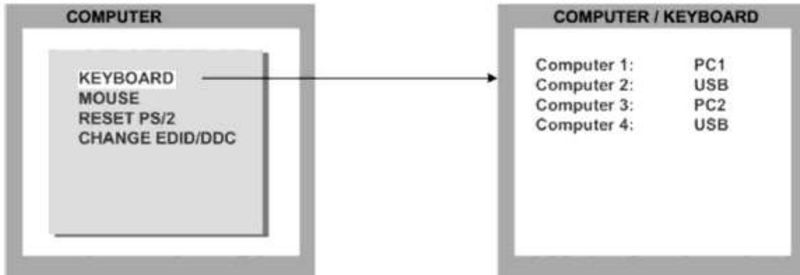
Use this display feature to identify which keyboard type (USB, PC1, PC2 or PC3) has been recognized at which computer port.
