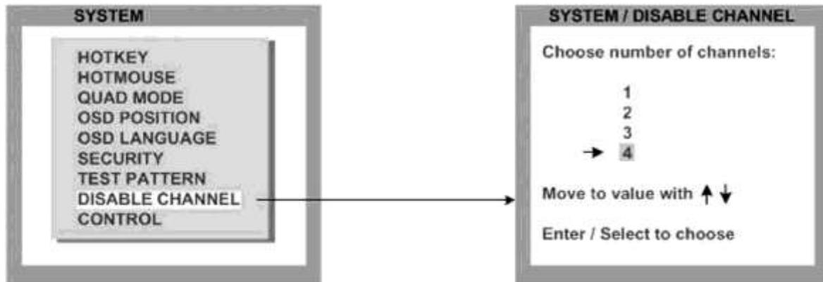
If only two or three computers or video sources are connected to KVMQUADPIP-4, use the DISABLE CHANNEL feature to ensure that for the unused channels:
