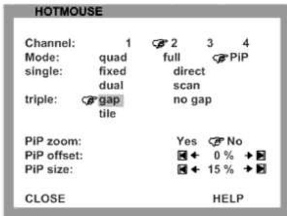
**Triple gap:** PiP images are displayed with a gap in place of the active channel.
