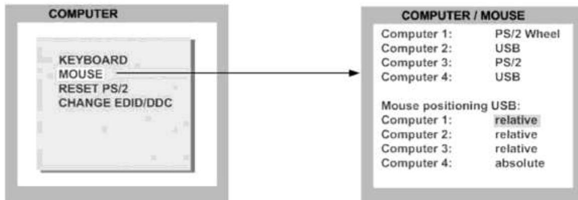
The upper half of the MOUSE window shows which mouse type (USB, PS/2 or PS/2 wheel) has been recognized at which computer port.
