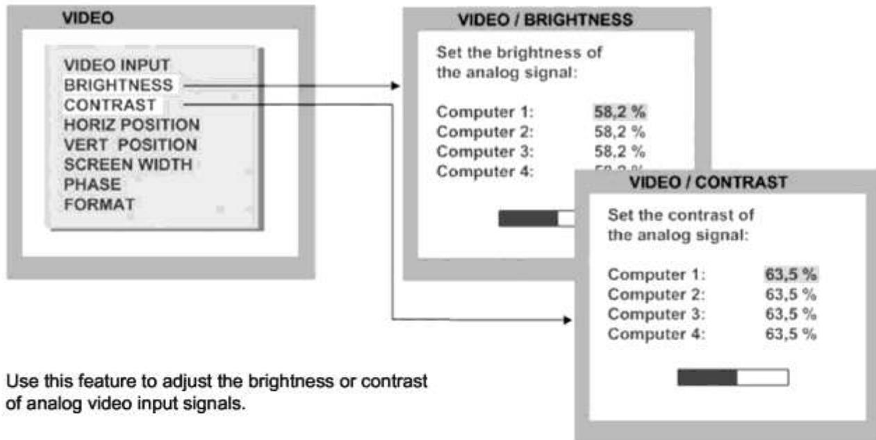
Use this feature to adjust the brightness or contrast of analog video input signals.
