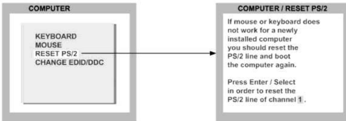
Use arrow keys ◀▶ or "+" and "-" keys to select the channel (1 to 4) you wish to reset and confirm by pressing ENTER/SELECT.
