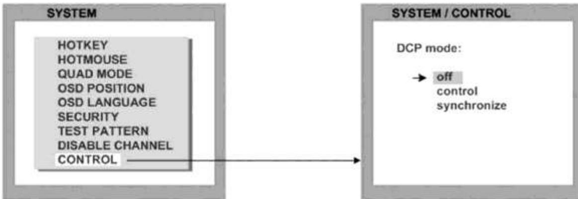
HETEC devices can be controlled via DCP (Device Control Protocol), an XML-based protocol. (See „DCP\_Manual.pdf“ on CD.)
