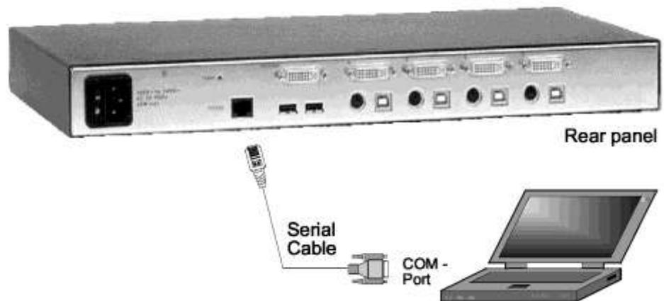
Use the serial cable to connect the COM port of the Windows computer with the serial port of your KVMQUADPIP-4.
