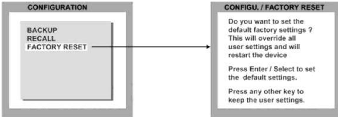
Use this function to reset the KVMQUADPIP-4 to its default settings. If necessary, save your current settings before using the DEFAULTS command. Execution of this command results in a complete reset and reboot of the KVMQUADPIP-4 with factory defaults.
