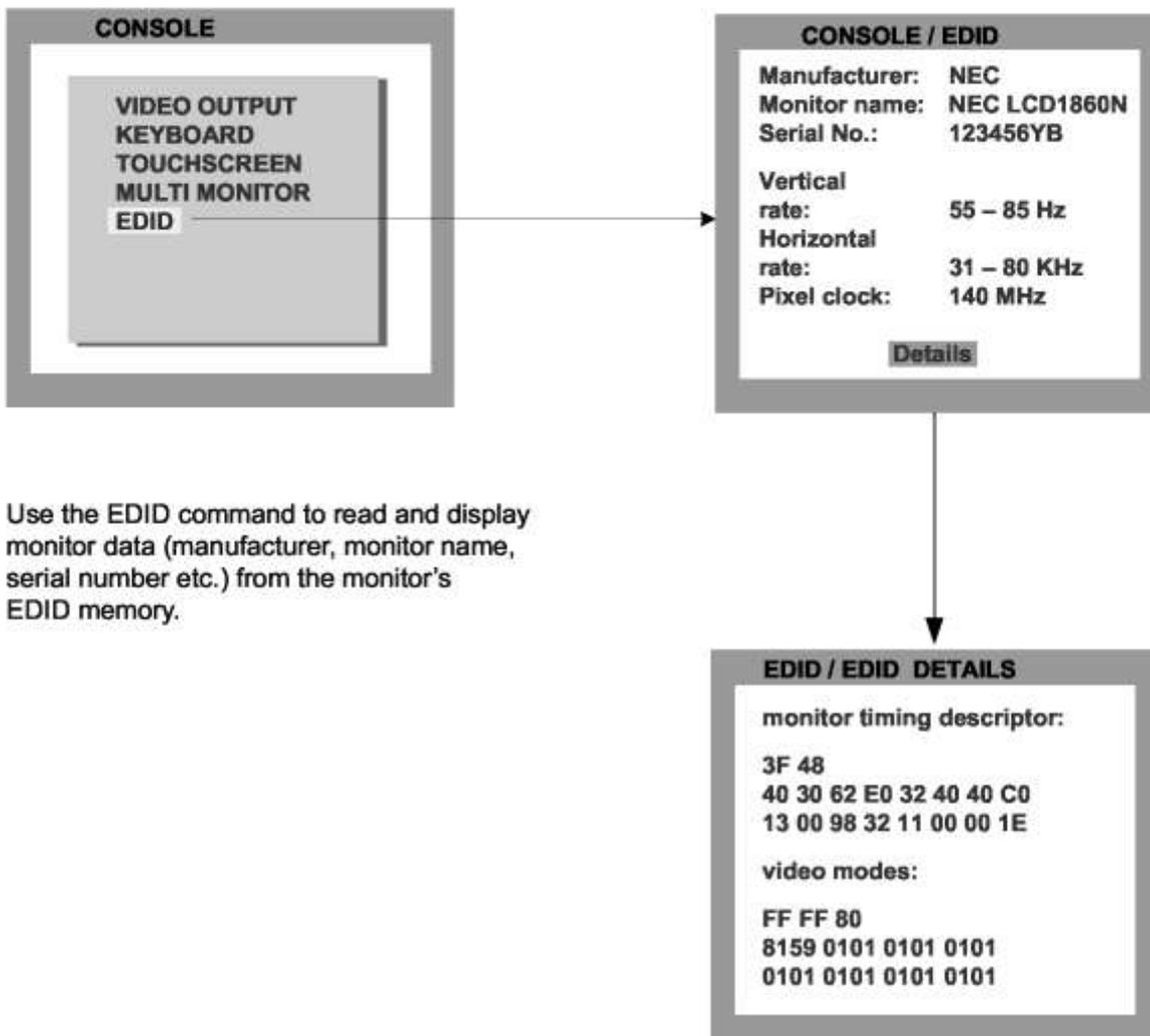
Use the EDID command to read and display monitor data (manufacturer, monitor name, serial number etc.) from the monitor's EDID memory.
