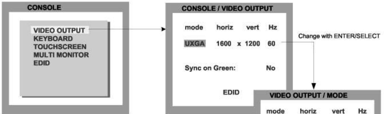
Use the VIDEO OUTPUT menu to choose an output resolution supported by your monitor. Press ENTER/SELECT to enter the selection menu. Use arrow keys to select the desired line in the list shown on the right and press ENTER/SELECT for the new video format.
