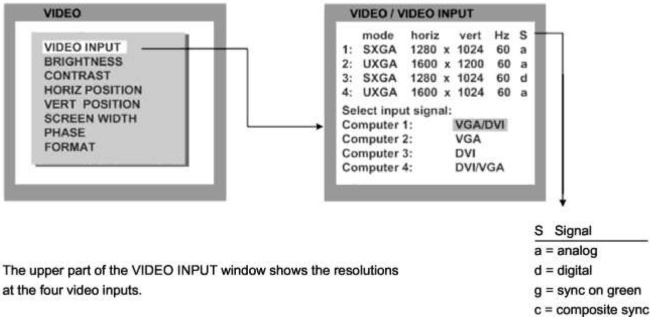
The upper part of the VIDEO INPUT window shows the resolutions at the four video inputs.
