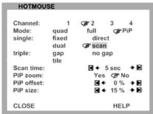
**Single scan:** Cycles through the PiP images at a set interval.
