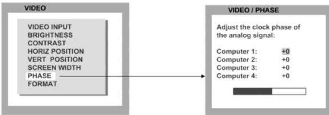
Incorrect phase (sampling time of pixel color value) may result in blurring, bad contrast, or poor legibility. Use this setting to adjust phase.
