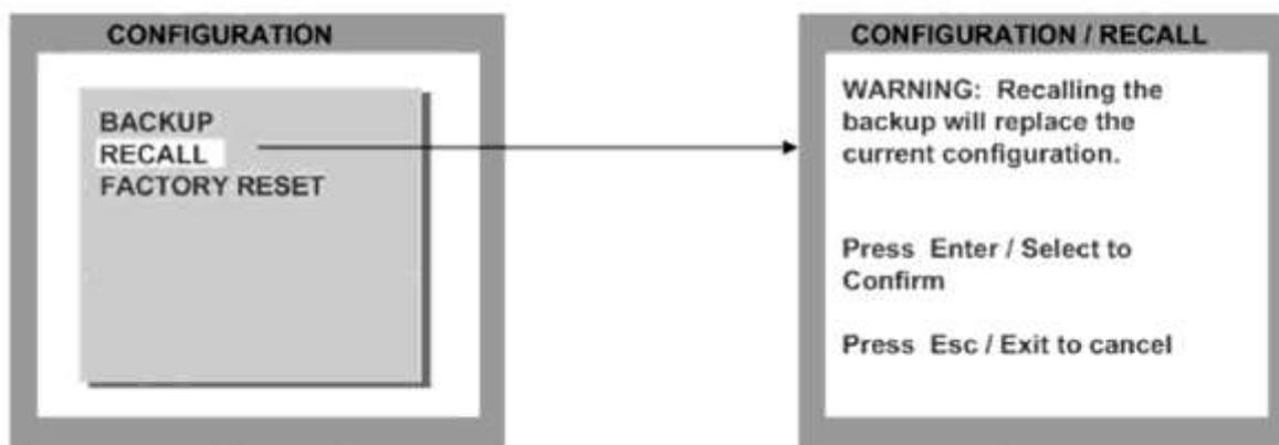
Use this feature to replace the current settings with the last configuration saved using the BACKUP command.
