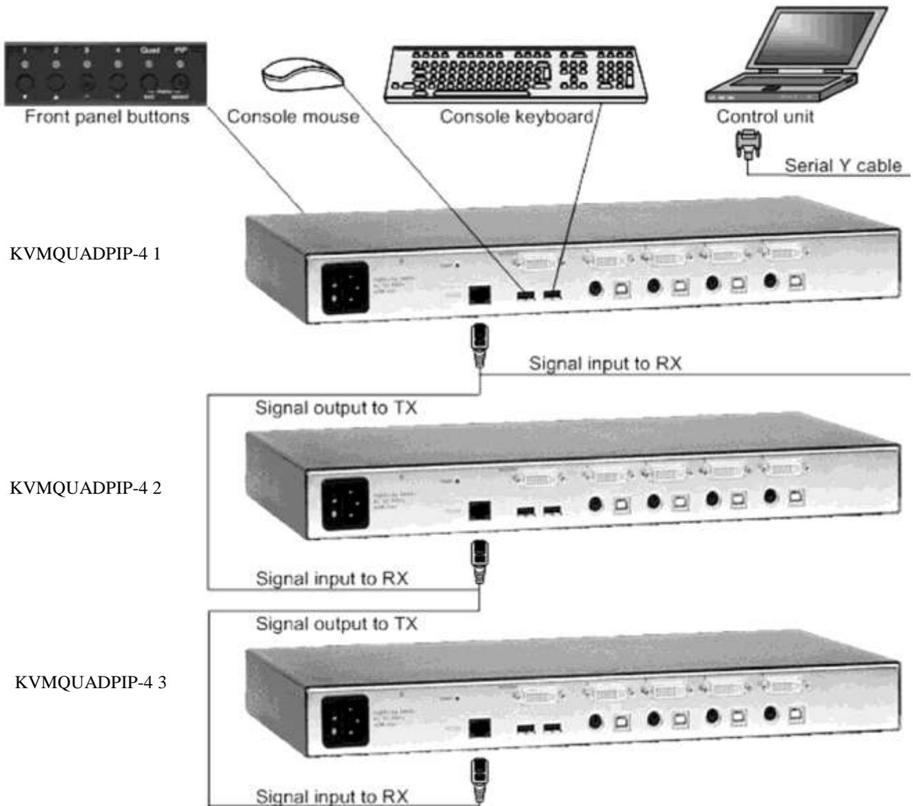
To synchronize, KVMQUADPIP-4 1 sends every change in settings as a DCP message via the serial Y cable to the RX input of KVMQUADPIP-4 2.
