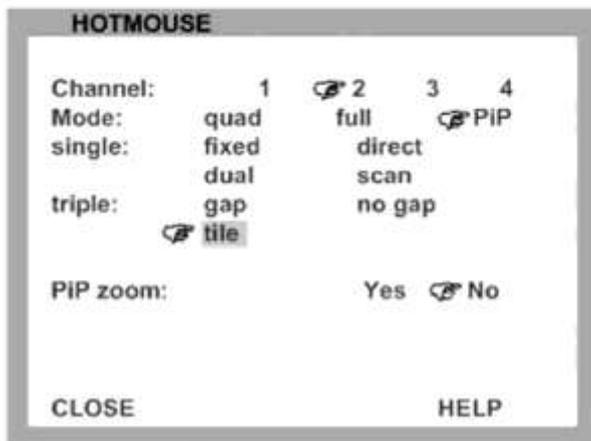
**Triple tile:** The size of the main image and the PiP images is optimized so that the main image and the PiP images are shown as large as possible without overlapping.
