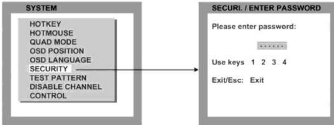
The SECURITY feature allows you to reduce the functional range of the KVMQUADPIP-4. Eight security levels are available for this purpose.
