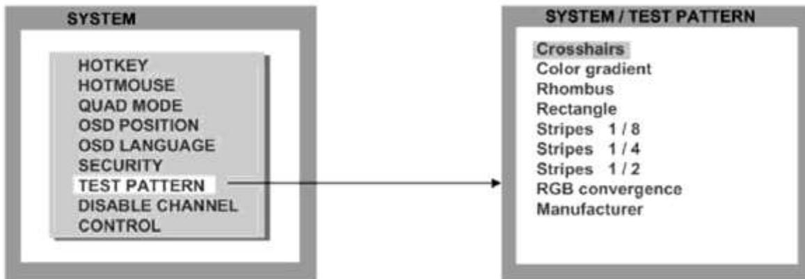
Use the Test Pattern feature to check monitor quality (pixel errors, contrast, etc) or the functionality of the V-Switch quad's video output.
