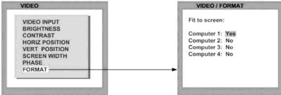
When using a wide-screen monitor (aspect ratio 16:10) in Quad-mode, a video input with a different aspect ratio is normally displayed with black borders to the left and right. If fit to screen is enabled, the image is resized to fill the entire quadrant in Quad mode.
